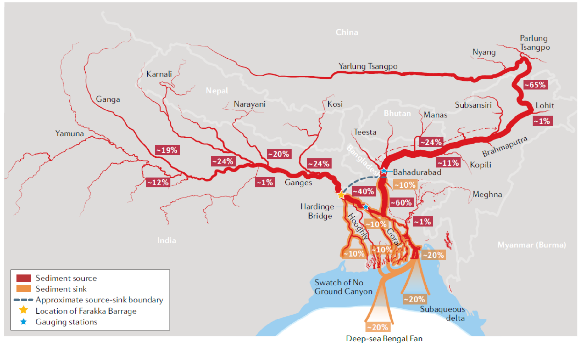
Fig. 4 | Sediment budget in the Ganges–Brahmaputra–Meghna delta system. Sources and sinks based on literature values 52,73,77,183–185 . Numbers represent percentage distributions of sediment entering (red) and leaving (orange) the delta, and dotted blue line represents the approximate location where the delta receives 100% of its sediment before depositing it downstream.
